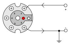
Use twisted pair or screened cables for cable lengths greater than 30 metres. Maximum cable length 1000 metres.
